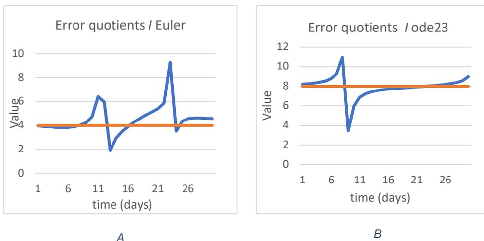
Figure 13: A and B show the plots of the error quotients for the Euler and ode23 solution for I.
